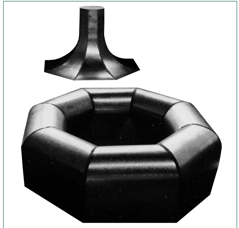
Photograph of axial inlet silencing components. Lower is the bellmouth inlet. Upper is the center body which is inserted in the bell mouth component (after the bellmouth is turned 180 degrees from the position shown).
